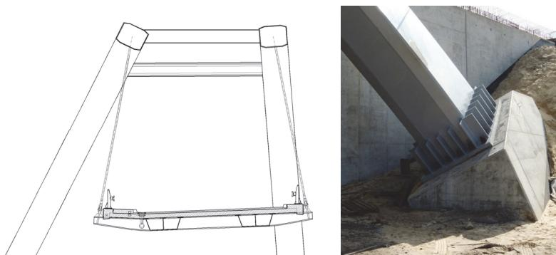
Figure 8: Cross-section and fixing of the arch in the abutment [4]
