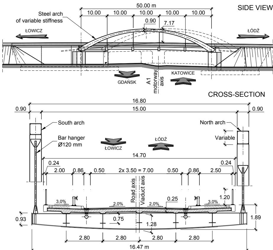
Figure 2: Side view of the viaduct in Stryków and cross-section of the span in the middle of the southern arch
