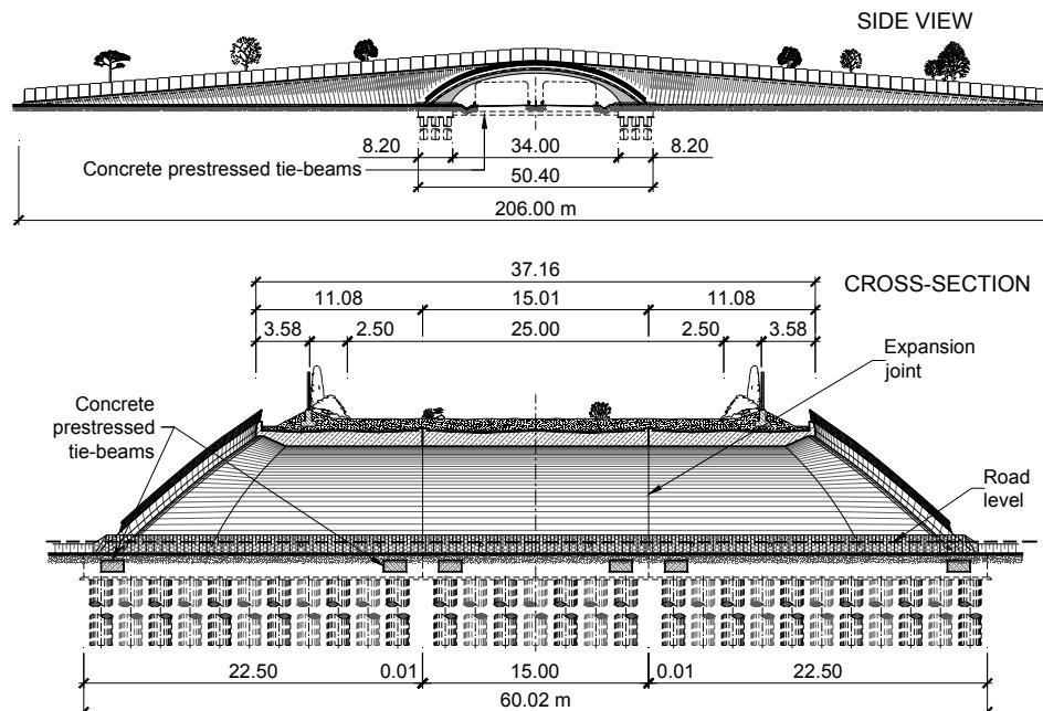
Figure 6: Side view and cross-section of the green viaduct
