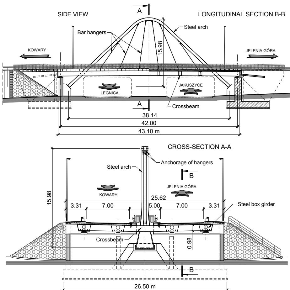
Figure 4: Side view and cross-section of the viaduct in Jelenia Góra
