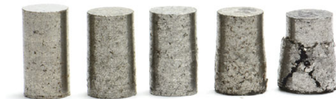
Fig. 19. Compression test cylinders before (left), during (middle) and after the test (right).
