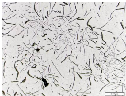
Fig. 16. Metallography of the cast iron material after embedding and polishing the surface.
