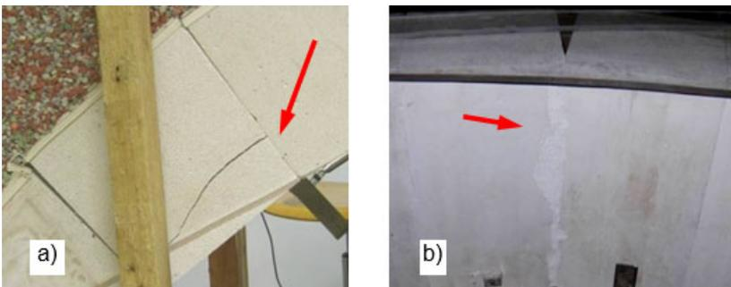
*Fig. 8. Deep ( $r/s = 0.3$ ) ARCH + FILL. a) left and b) right hinge (final stage).*
