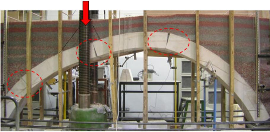
*Fig. 7. Collapse mechanism of 1the deep ( $r/s = 0.3$ ) Arch + Fill.*
