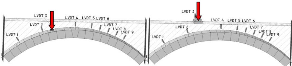
Fig. 2. Load directly on the arch and load on the fill surface.
