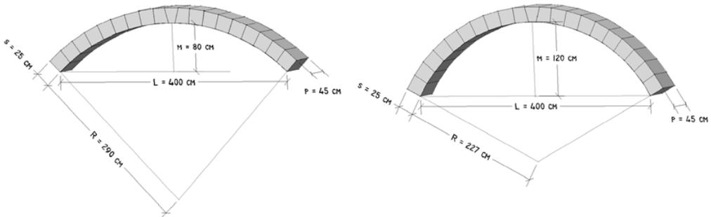
Fig. 1. Shallow arch.  $r/s = 0.2$  and deep arch.  $r/s = 0.3$ .
