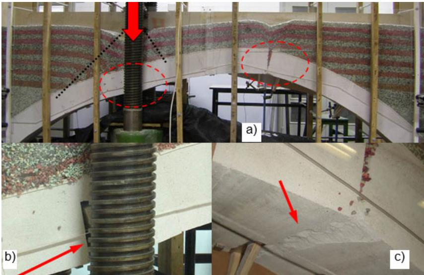
**Fig. 5.** Collapse mechanism of the shallow ( $r/s = 0.2$ ) ARCH + FILL. a) global mechanism; b) left and c) right hinge (final stage).
