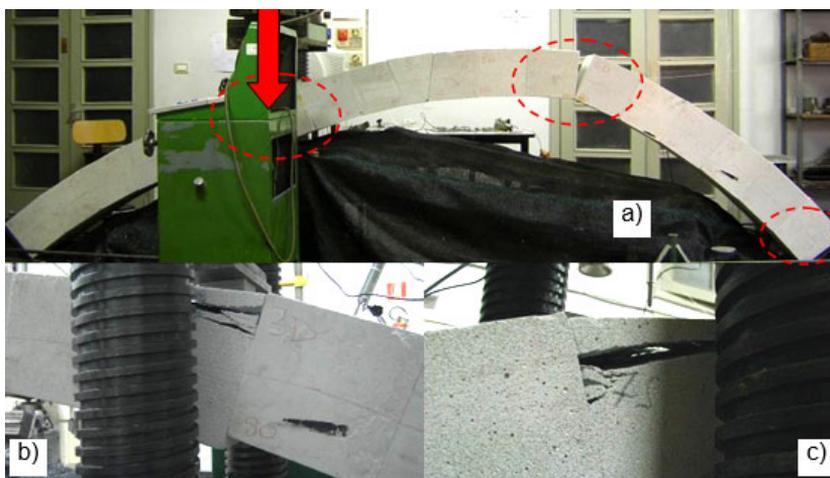
**Fig. 4.** Collapse mechanism of the SHALLOW ( $r/s = 0.2$ ) ARCH. a) global mechanism; b) and c): details of the “hinge” just below the load (final stage).
