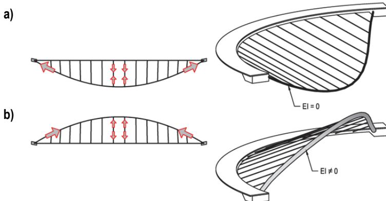
Figure 8: Form finding – a) suspension structure, b) arch structure
