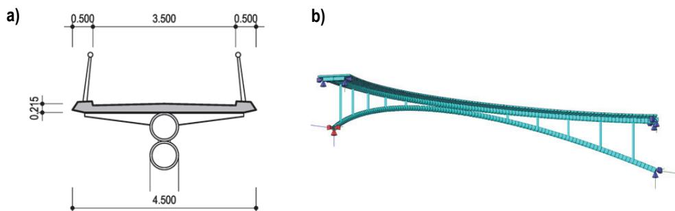
Figure 5: Bridge supported by the curved arch – a) cross section, b) calculation model
