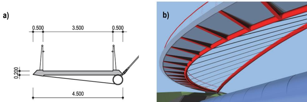
Figure 6: Bridge deck – a) cross section, b) visualization
