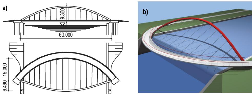
Figure 7: Bridge suspended on the arch – a) elevation and plan, b) visualization
