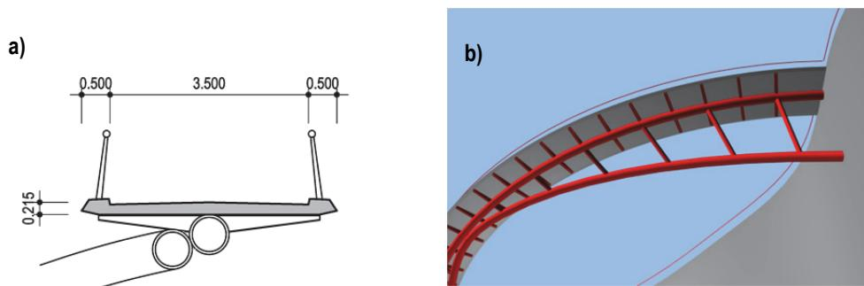
Figure 9: Bridge deck – a) cross section, b) visualization
