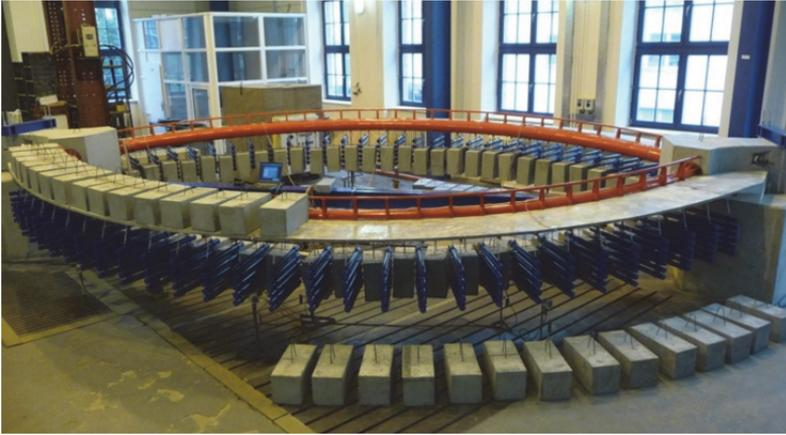
Figure 1: Model test of the curved stress ribbon & flat arch structure
