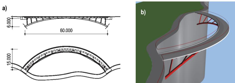
Figure 10: Bridge supported by the arch – a) elevation and plan, b) visualization
