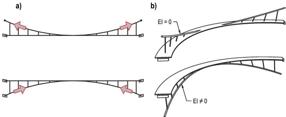
Figure 11: Form finding – a) suspension structure, b) arch structure
