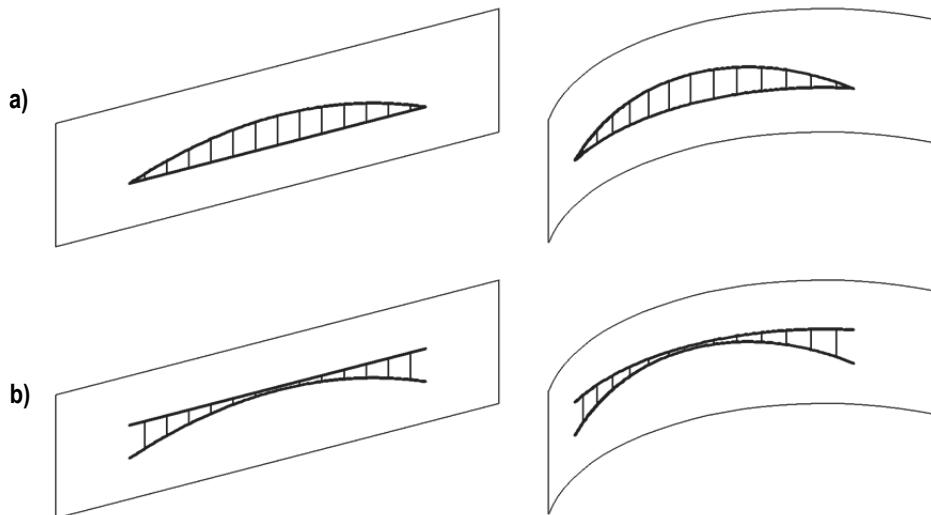
Figure 3: Plan curved bridge suspended (a) or supported (b) by a curved arch
