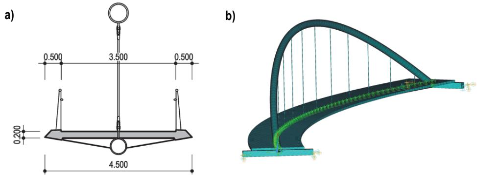
Figure 4: Bridge suspended on the curved arch – a) cross section, b) calculation model
