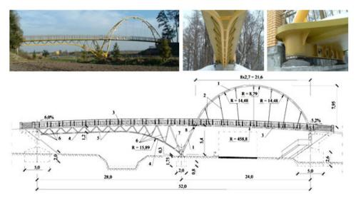
**Fig. 3.** Arch footbridge in Bieruń Stary, Poland (Engineering Studio Project s.c.): 1 – steel tube Ø244.5/8 mm; 2 – steel bar Ø30 mm; 3 – steel box-girder filled with concrete (steel plate 6 mm thick); 4 – steel tube Ø193.7/14.2 mm; 5 – steel tube Ø101.6/7.1 mm; 6 – steel tube Ø108.0/8.0 mm; 7 – steel tube Ø168.3/12.5 mm; 8 – hinged connection constructed using elastomeric bearing placed in steel tubes.
