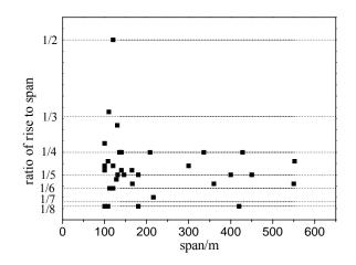
Figure 4 : relationship between ratio of rise to span and span
