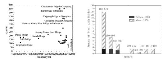
Figure 1 : span and finished year of steel arch bridge
