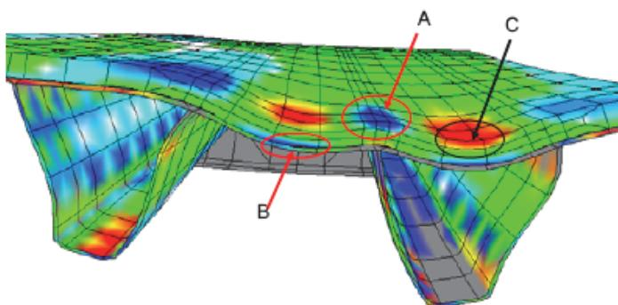
Figure 1: Stresses in the cross section of an orthotropic steel bridge
