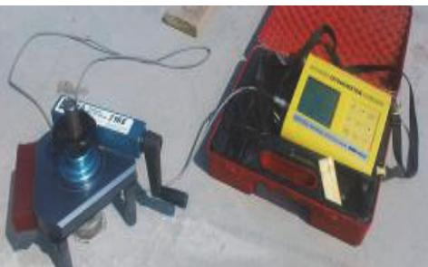
Figure 4: Adhesion testing device
