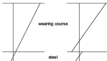
Figure 2: Assumed stress distributions within the cross section of the bridge
