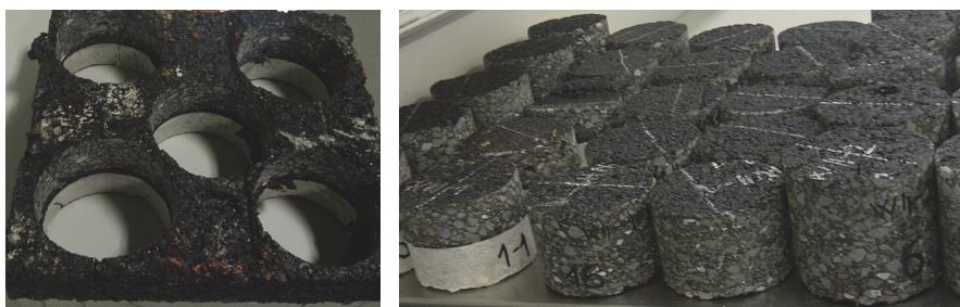
Figure 5: Drilled cores of the system for testing of layers cohesion
