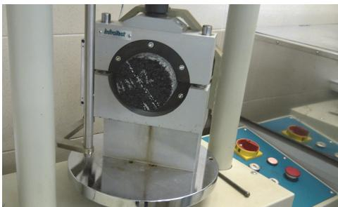
Figure 3: Testing of layers bond
