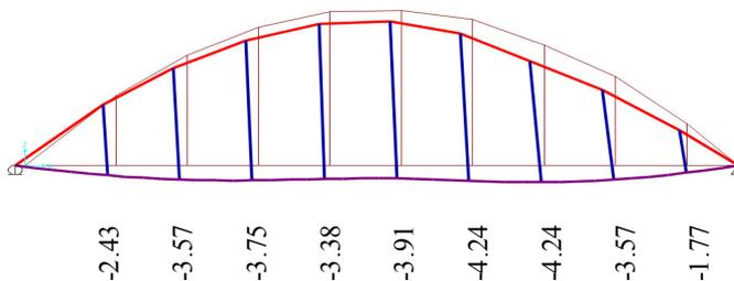
Fig. 10. Live load deflection of arch girder.
