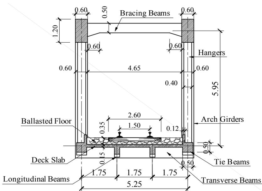
Fig. 3. The bridge cross sectional dimensions.
