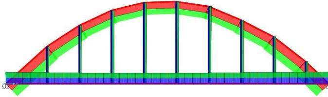
Fig. 8. Ultimate axial forces of arch girders, ties, and hangers.
