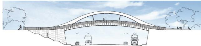
Figure 8: Elevation of the footbridge in its context
