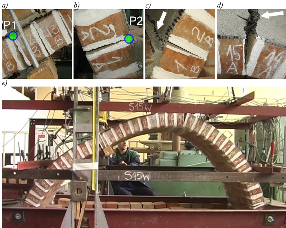
Fig. 5. Arch VC-An (originally named S15W): a)-d) cracks and hinges of the collapse mode, e) failure mechanism.
