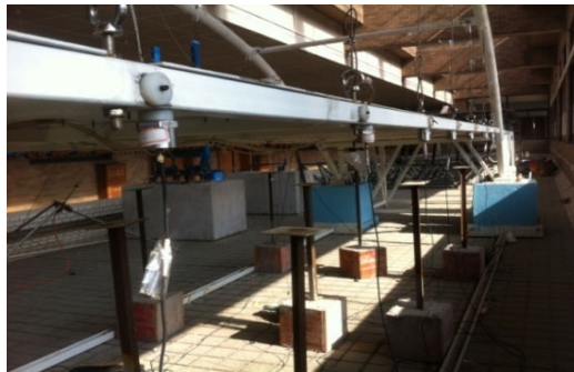
c) arrangement of acceleration sensors in vertical and transverse direction for the deck.
