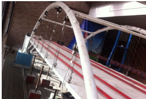
b) arrangement of acceleration sensors in vertical and transverse direction for the arch ribs.
