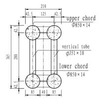
Fig. 4: Cross section of arch rib
