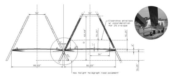
Figure 8 : Unequal Length of arches
