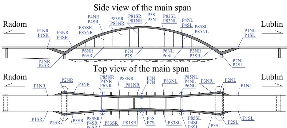
Figure 1: Position of test points on the bridge in Puławy
