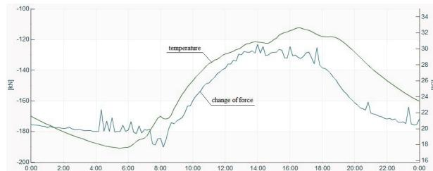
Figure 2: Change of forces and the temperature of central hanger, 12.08.2010
