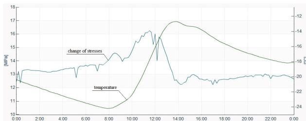
Figure 4: Change of stresses and the temperature of the arch at the point P5N, 26.01.2010
