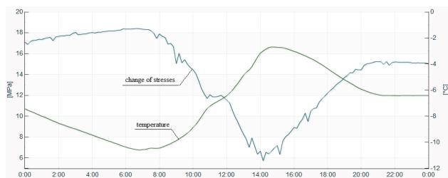
Figure 5: Change of stresses and the temperature of the arch in point P3NR, 08.03.2010
