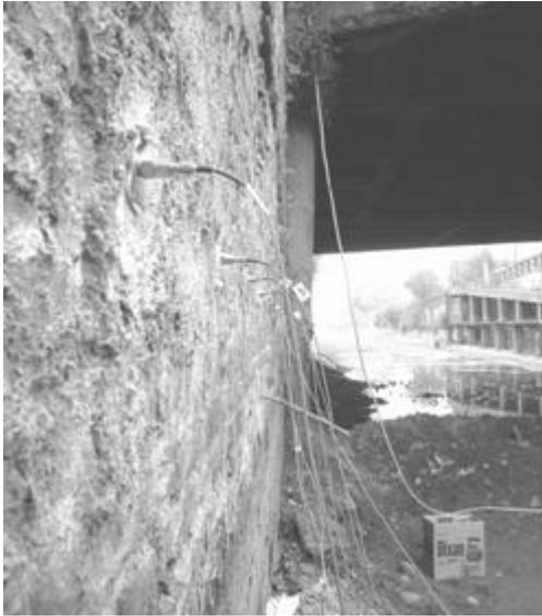
Figure 9. Accelerometers installation
