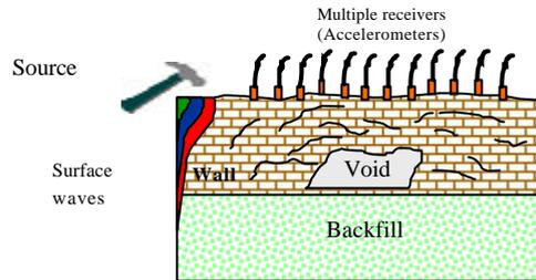
Figure 6: Example of multi-channel array of transducers
