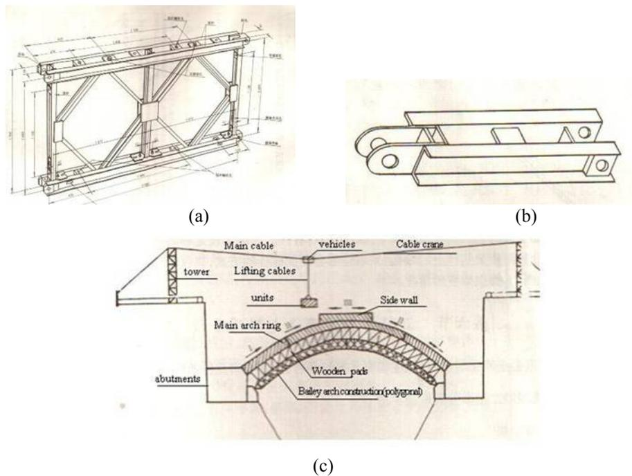
Figure 2 : Bailey arch construction in Guangdong Province:(a) Military prefabricated "Bailey truss beam, (b) Special component as a joint, (c) Schematic diagram of casting the main arch ring on Bailey arch construction
