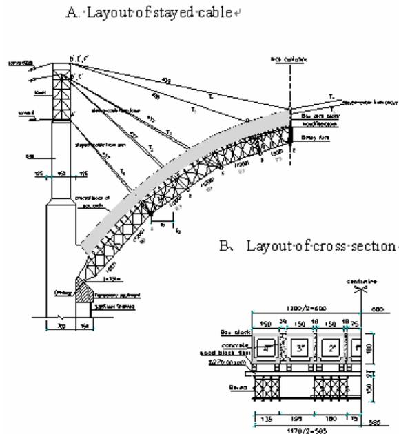
Figure 3 : 133m-long Cable-stayed Bailey Steel Arch Construction
