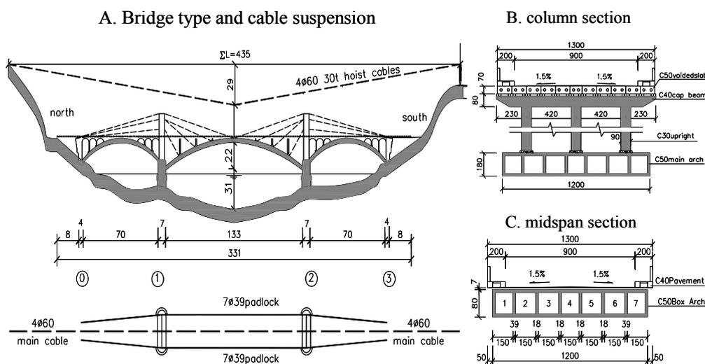
Figure 1 : Construction of Hunan Wuqiangxi Hydropower Station Ruanshui Bridge Figure
