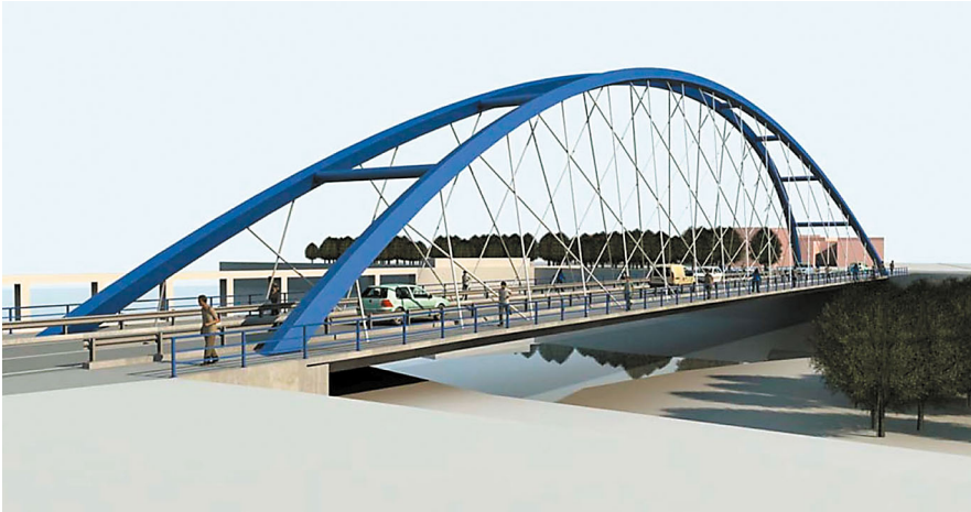
Fig. 15. Model of the bridge, showing the arches, bracing and network.
