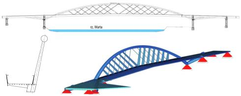
Fig. 3. Modified design. Elevation, cross section and FEM SOFiSTiK model.
