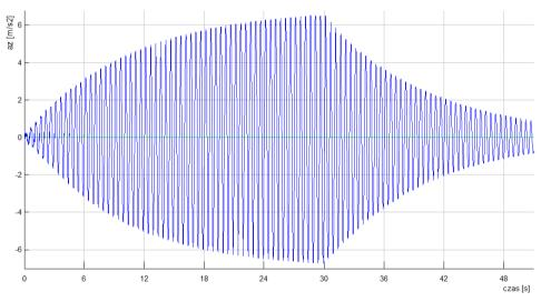
Fig. 6. Max. vertical acceleration on deck – test C5 – max=6.515 [m/s2].
