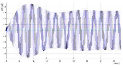
Fig. 5. Test Pf3 max. vertical acceleration of the deck – stabilization  $\sim 1 \text{ [m/s2]}$ .
