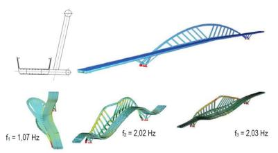
Fig. 2. Original FEM SOFiSTiK model, cross section and first three eigen forms and frequencies.
