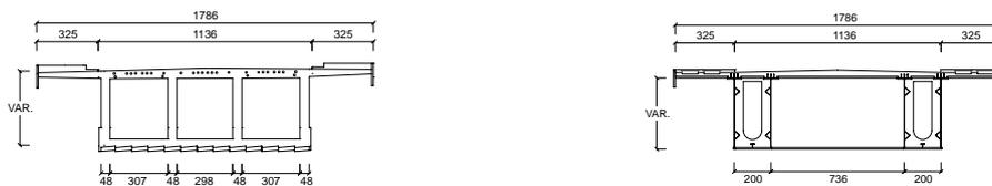
Figure 3 : Typical cross section of original solution    Figure 4 : Typical cross section of updated solution
