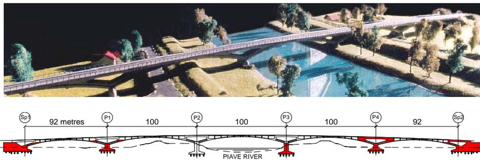
Figure 1 : The original solution as planned and as built (in red hatch) before work interruption
