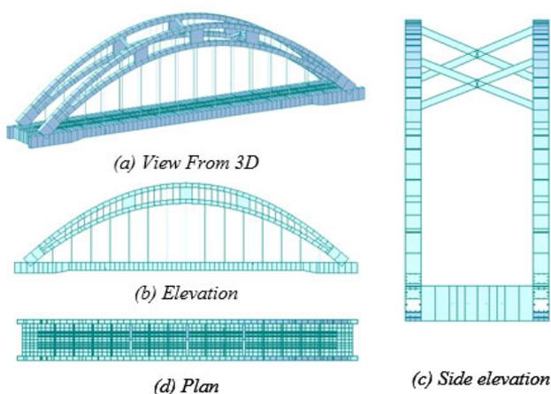
Fig. 3. Finite element model of Xinkai River Bridge.
