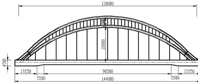
Fig. 2. Elevation of Xinkai River Bridge (mm).
