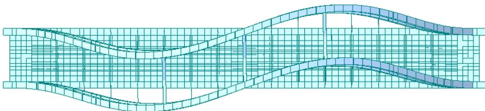
*Fig. 5. The first order buckling mode of Xinkai River Bridge.*
