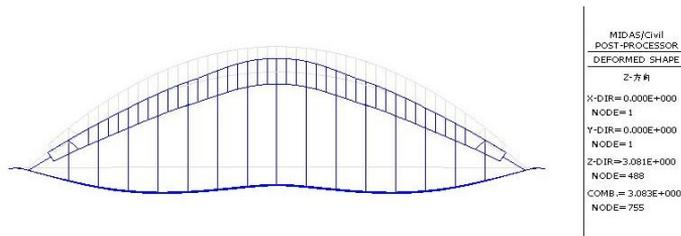
Fig. 4. Vertical deflection of arch bridge.
