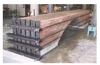
Fig. 2. Steel plates confining the infill and the ties balancing the plates.
