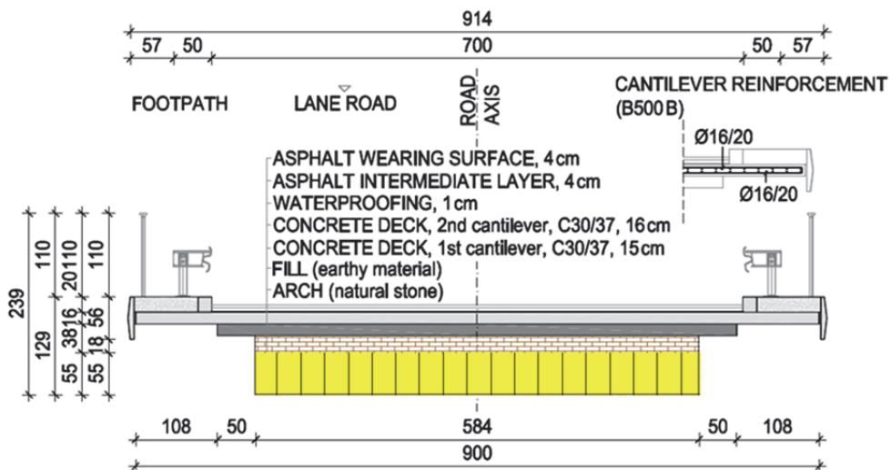
Figure 6: Cross-section of a proposed new bridge deck
