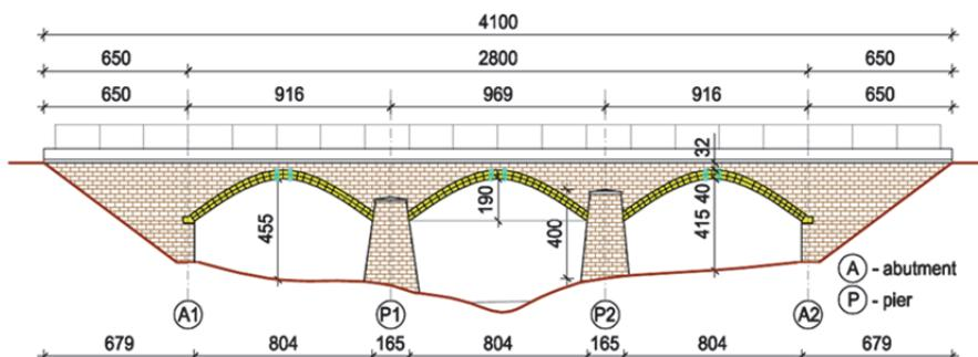
Figure 2: Longitudinal disposition of the bridge
