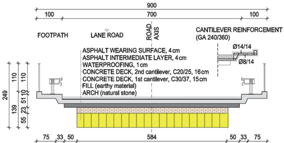
Figure 4: Cross-section of the existing bridge
