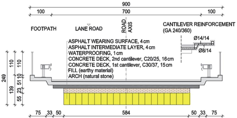
Figure 4: Cross-section of the existing bridge
