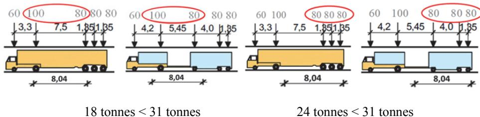
Figure 5: Influence of axle distances of the axle loads of the representative vehicles (tug trucks) and 6 (trucks with trailers) acting on the bridge span
