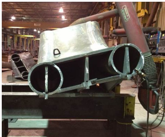
Fig. 5. Centre arch knuckle fabrication.
