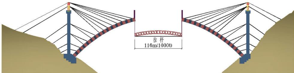
Figure 17: Construction diagram of combination method
