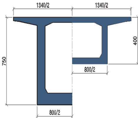
Figure 11: Typical section of (2-60m) T-type frame structure (unit: cm)
