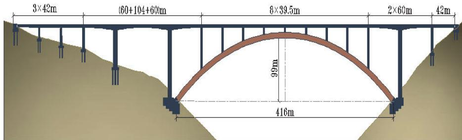
Figure 5: General layout of deck concrete whole-box arch
