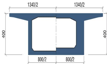
Figure 12: Typical section of (8-39.5m) continuous beam (unit: cm)
