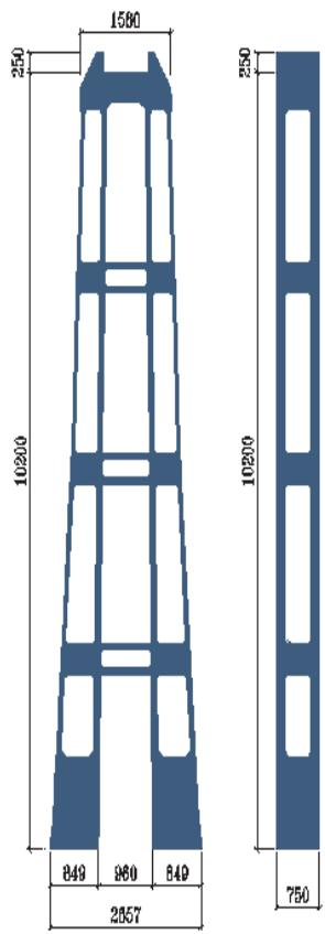
Figure 9: Junction pier (unit: cm)
