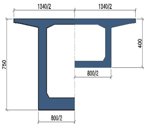
Figure 11: Typical section of (2-60m)
