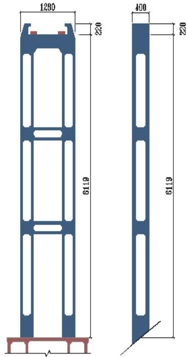
Figure 10: No.1 spandrel column (unit: cm)
