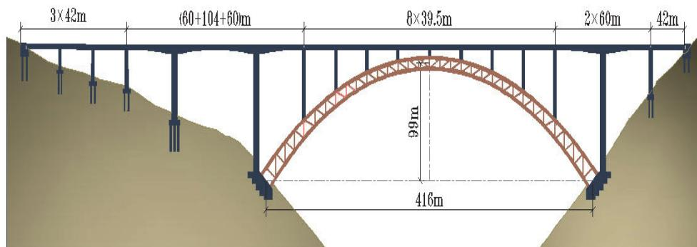
Figure 2: General layout of deck steel truss arch
