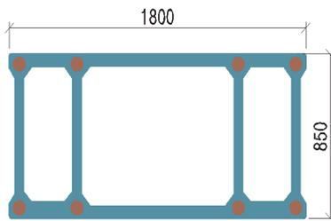
Figure 7: Arch section at the arch crown (unit: cm)
