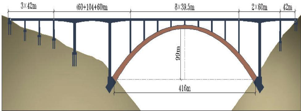
Figure 4: General layout of deck concrete twin-rib arch
