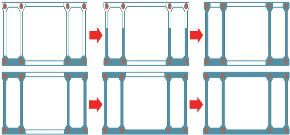
Figure 16: Construction diagram of casting the arch ring concrete
