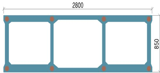
Figure 8: Arch section at the arch springing (unit: cm)
