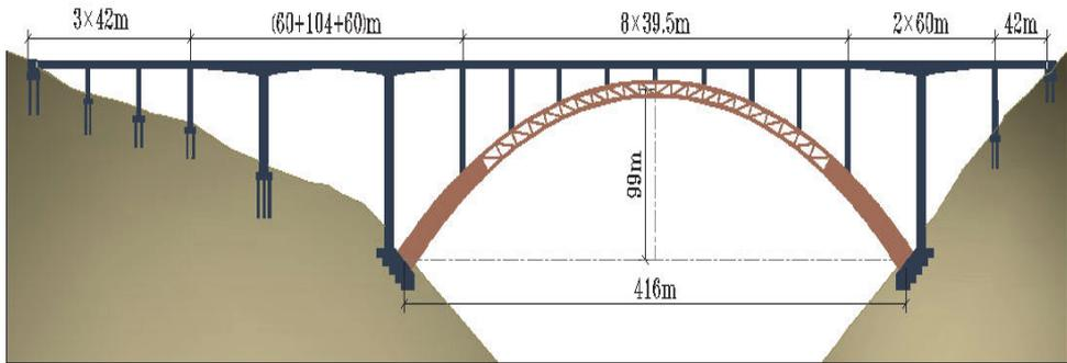
Figure 3: General layout of deck CFST arch
