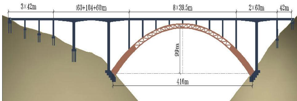
Figure 3: General layout of deck CFST arch
