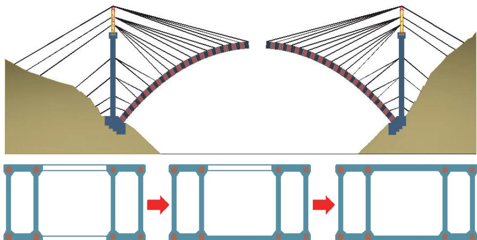
Figure 13: Schematic diagram of cable-stayed cantilever erection method
