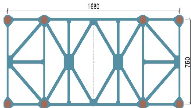
Figure 14: Cross section of steel tubular truss at the arch crown (unit: cm)
