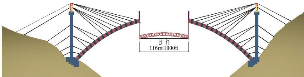
Figure 17: Construction diagram of combination method
