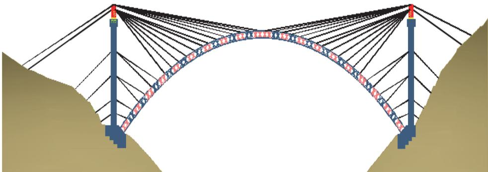
Figure 15: Construction diagram of erecting steel tubular truss
