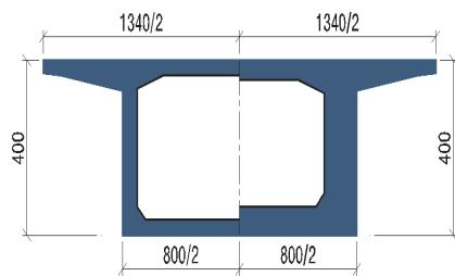
Figure 12: Typical section of (8-39.5m)
