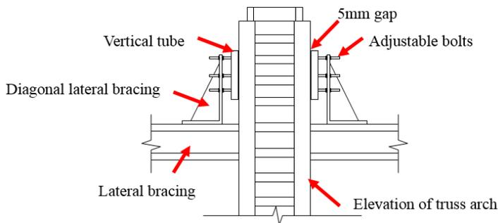
*Fig. 4. Anti-laterally overturning device.*
