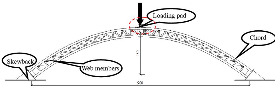
Fig. 1. Plan view of CFST truss arch model (A-0, Units: cm).
