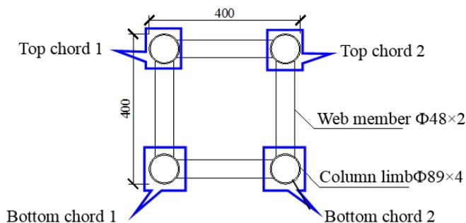
Fig. 2. Cross-section of arch rib (unit: mm).
