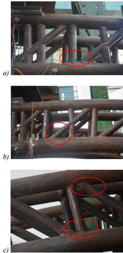
**Fig. 4.** Failure photos of web braces of A-0:
