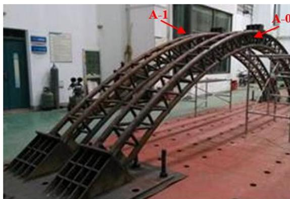
Fig. 3. Photos of CFST truss arch model.
