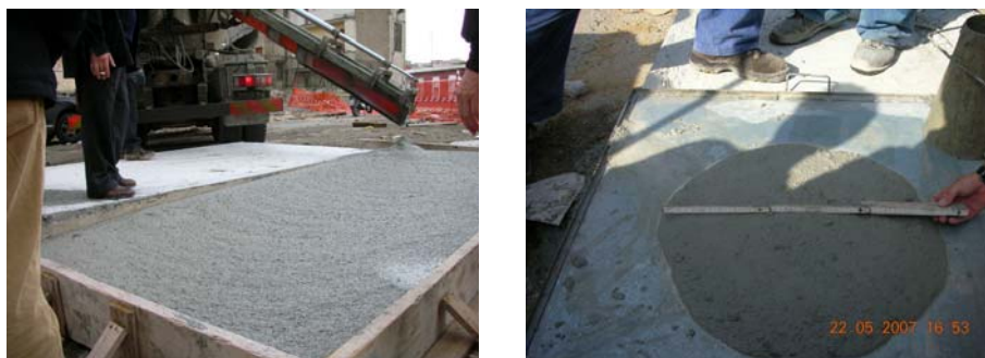
Figure 5 : Special testing for checking viscosity on an inclined plane and slump flow test for SCC
