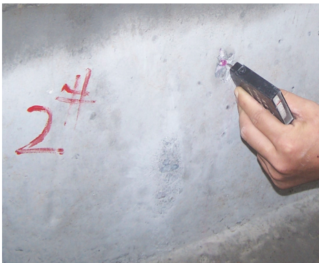
Figure 2: Concrete Carbonation Test (2006) Figure 3: Bridge Deck System Disease (2007)
