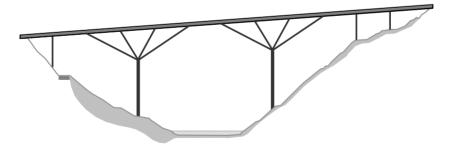
Fig. 4: Alternative B - Continuous beam upon a "tree" structure
