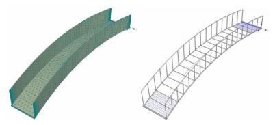
Fig. 5. Finite element mesh on the left and on the right: Segmentation of macroelements to surfaces and reinforcement of the anchoring area.
