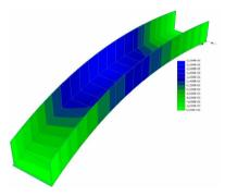
Fig. 6. Vertical deflection of the structure before failure, the applied force of  $18.9 \text{ kN/m}^2$ , the maximum deflection value -22.59 mm.
