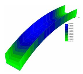
Fig. 8. Vertical deflection of the structure, the applied force of 4,2 kN  $/m^2$ , the maximum deflection value -2.66 mm.
