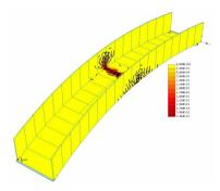
Fig. 7. Cracks on the structure prior to the failure, the applied force of  $18.9 \text{ kN}/\text{m}^2$ , the maximum crack width 3.18 mm.
