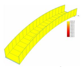
*Fig. 9.* Cracks on the structure, the applied force of  $4,2 \text{ kN/m}^2$ , the maximum crack width 0,0006 mm.
