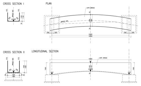
Fig. 4. Plan, longitudinal and cross section of the bridge.
