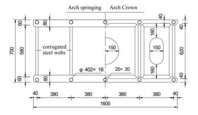
Figure 2: Arch cross section of of the trial designed bridge (unit: cm)
