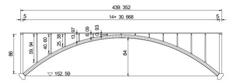
Figure 1 : Layout of the trial design (unit: m)
