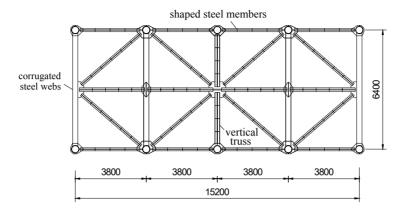
Figure 4 : Cross section of embedded scaffolding
