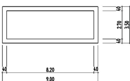
Pier Section at Axes 1, 2, 10-13
