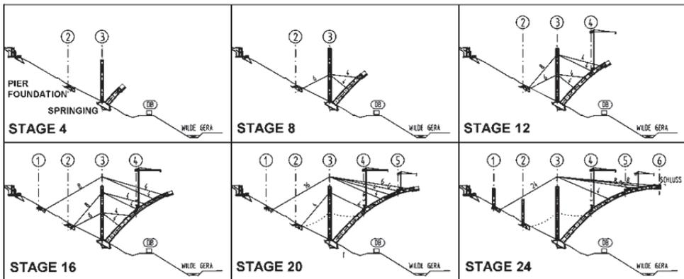
Figure 5: Stages of construction for one half of the arch
