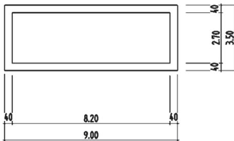
**Pier Section at Axes 1, 2, 10-13**
