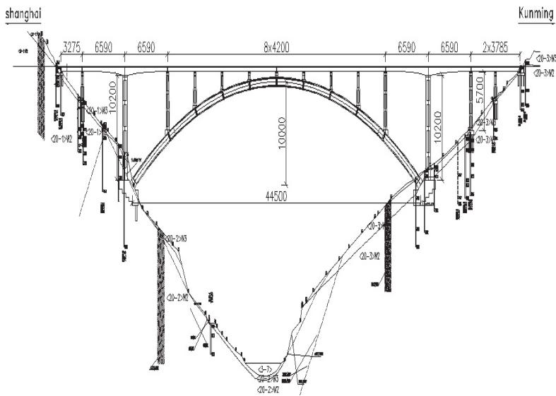
Figure 9: General layout of deck reinforced concrete arch bridge at the middle line level (unit:cm)
