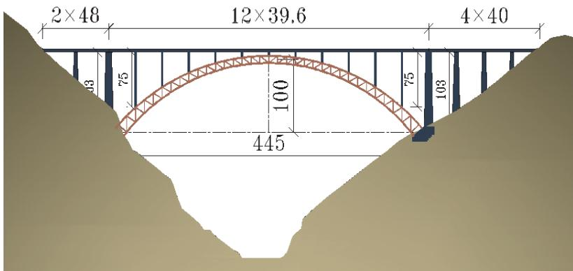
Figure 8: General layout of deck steel truss arch ( Unit: m)
