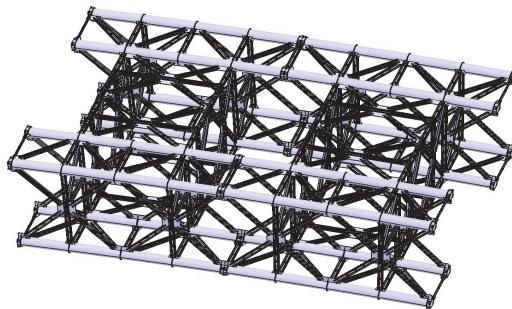
Figure 13: Segmental model of steel tubular truss by CATIA
