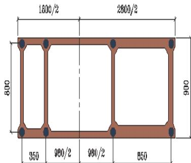
Half arch crown section    Half arch Springer section
