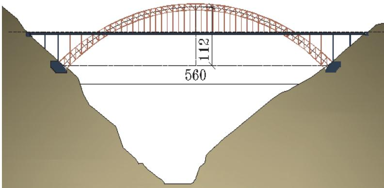
Figure 7: General layout of half through steel truss arch (Unit: m)
