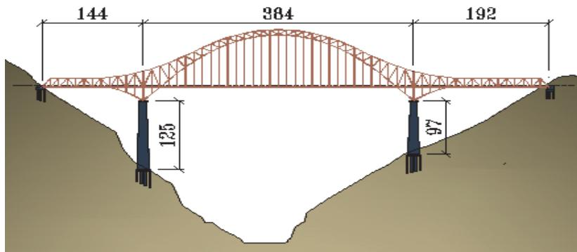
Figure 6: General layout of through steel truss arch (Unit: m)
