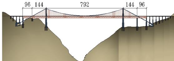
Figure 2: General layout of the suspension bridge for high line level
