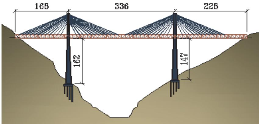
Figure 5: General layout of the cable-stayed bridge ( Unit: m)
