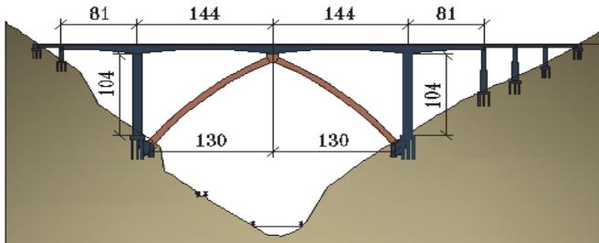
Figure 4: General layout of inclined leg arch bridge (unit: m)
