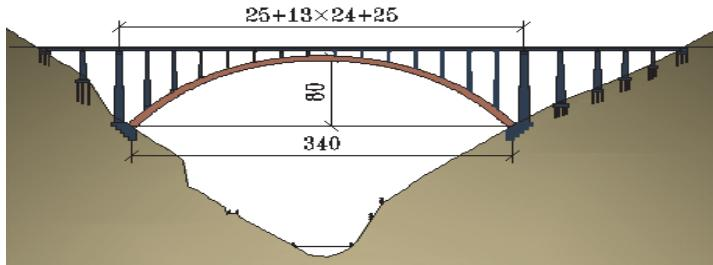
Figure 3: General layout of deck reinforced concrete arch bridge (unit: m)
