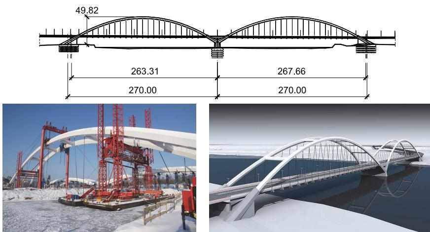
Figure 6: Side view, assembly of the arches (photo: K. Jędrzejewski – Strabag) and computer image of the bridge in Toruń [7]
