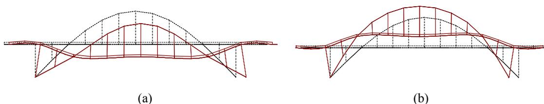
Figure 7 : Deformation modes of theoretical model in longitudinal direction. Direction:(a)Longitudinal direction(Shrinking), (b)Longitudinal direction(Expanding)
