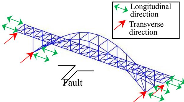
Figure 4 : Loading conditions in seismic fault displacement analysis
