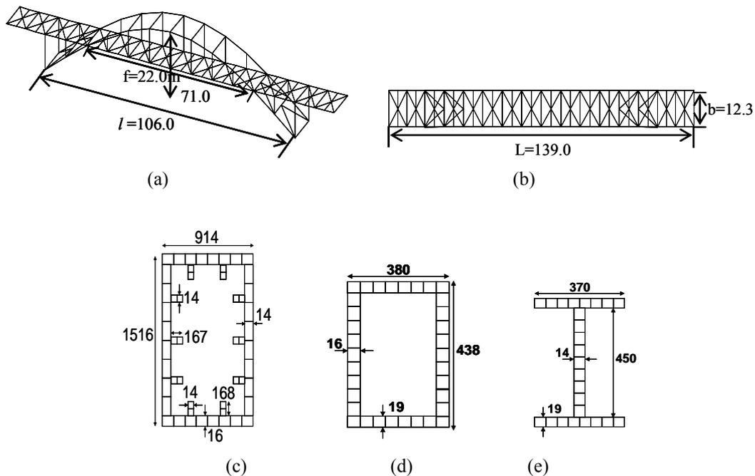
Figure 2 : Theoretical arch model (unit: m):(a)Global view of theoretical model, (b)Plane view of theoretical model, (c)Arch rib, (d)Vertical column, (e)Lateral member
