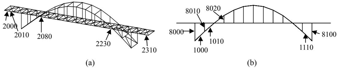
Figure 9 : Main element numbers of theoretical models in the arch direction (a) Arch rib and vertical columns, (b) Stiffened
