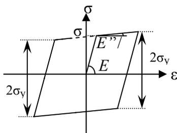
Figure 12 : Stress-strain relation of BRB
