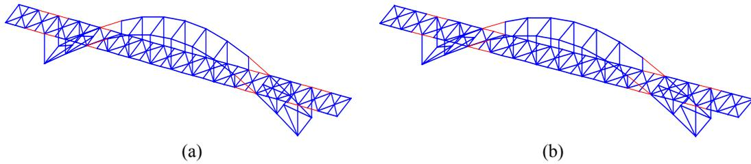
Figure 8 : Distributions of longitudinal strain in the arch direction:(a) Longitudinal direction(Shrinking), (b)Longitudinal direction(Expanding)
