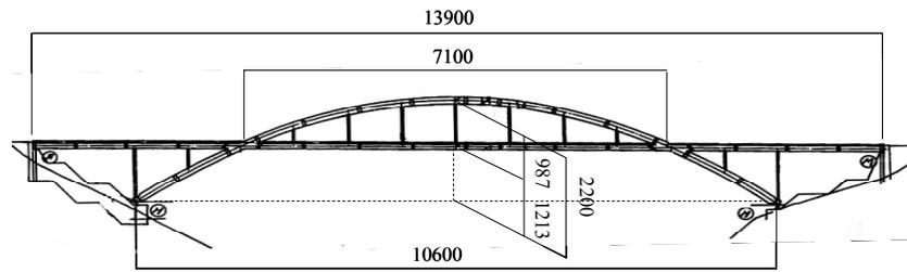
Figure 1 : Half-through arch bridge (unit: mm)
