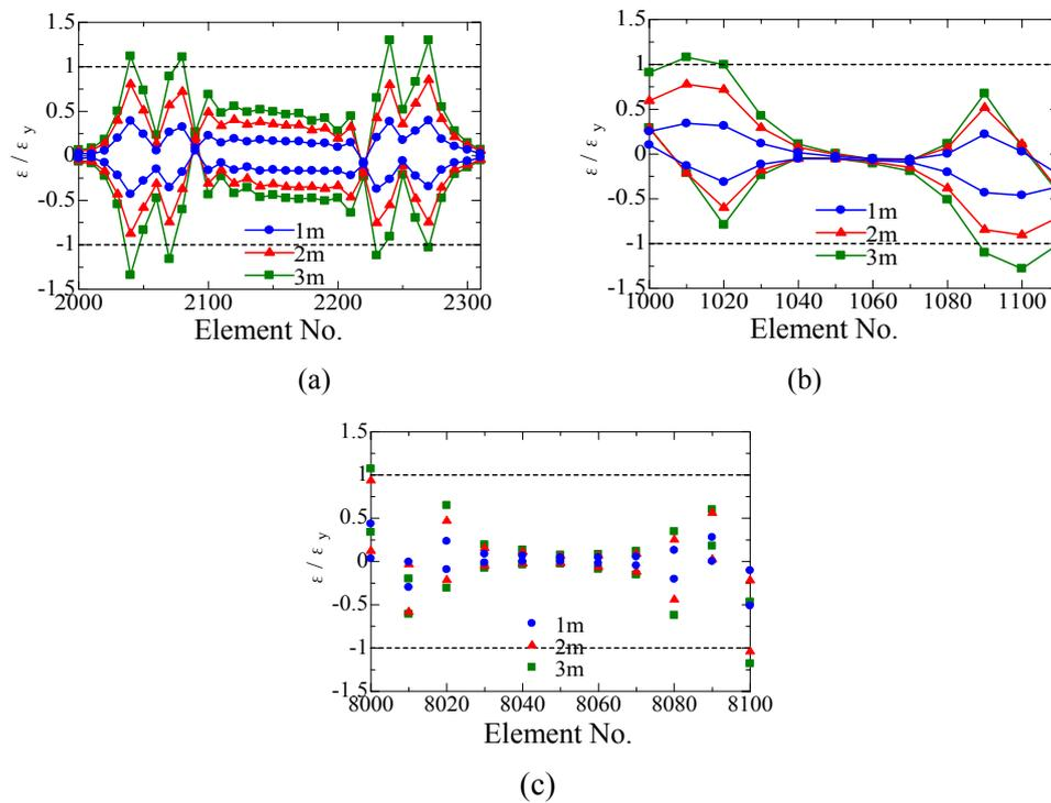
Figure 11 : Distributions of maximum and minimum plastic ratios of strain response in transverse direction:(a)Arch rib, (b)Stiffened girder, (c)Vertical column
