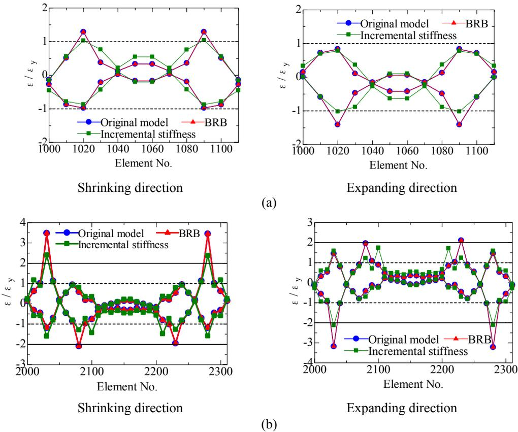
Figure 15 : Distributions of maximum and minimum plastic ratios of strain response in longitudinal direction : (a) Arch rib, (b) Stiffened girder
