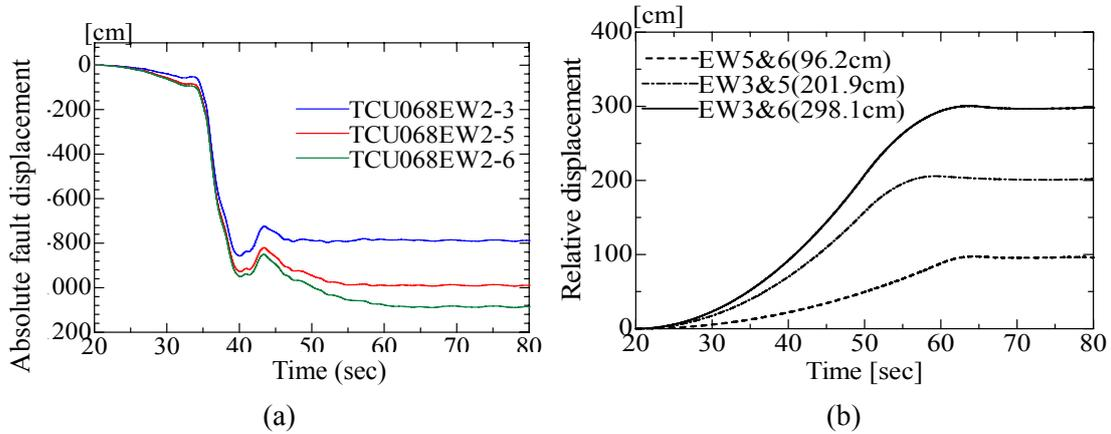
Figure 6 : Input fault displacement wave:(a)Input fault displacement wave, (b)Relative displacement
