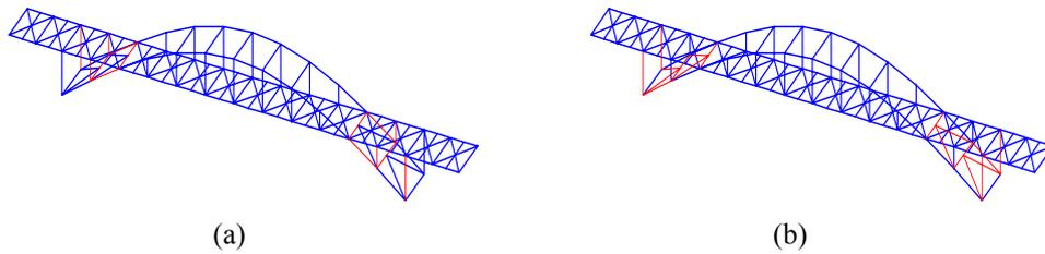
Figure 14 : Yield members in transverse direction (3m) : (a)BRB model, (b) Incremental stiffness model
