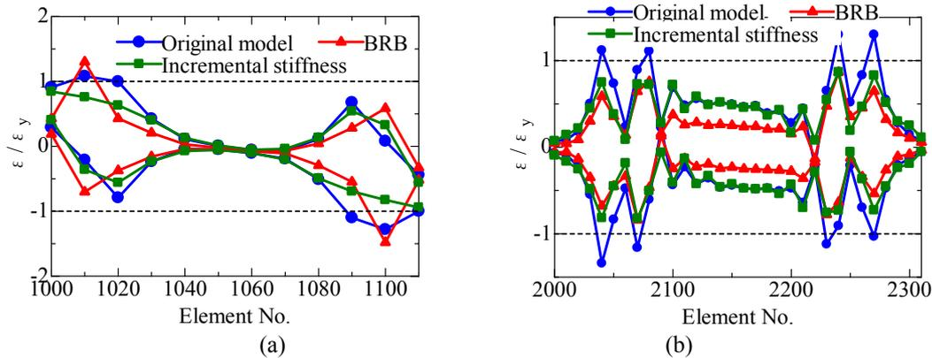
Figure 16 : Distributions of maximum and minimum plastic ratios of strain response in transverse direction
