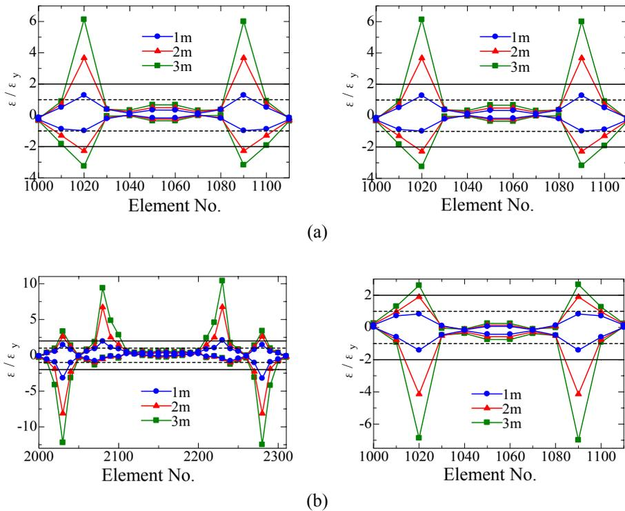
Figure 10 : Distribution of maximum and minimum plastic ratios of strain response in longitudinal direction : (a) Longitudinal direction (shrinking), (b) Longitudinal direction (expanding)
