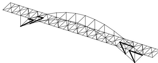
Figure 13 : Installed positions of BRB
