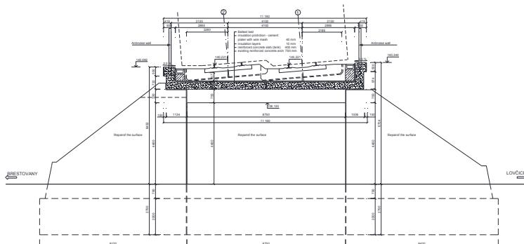
Figure 5: Reconstruction of arch bridge – cross-section
