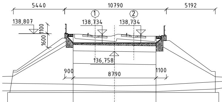
Figure 2: Reconstruction of arch bridge – cross-section
