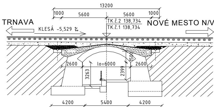
Figure 1: Reconstruction of arch bridge – longitudinal section
