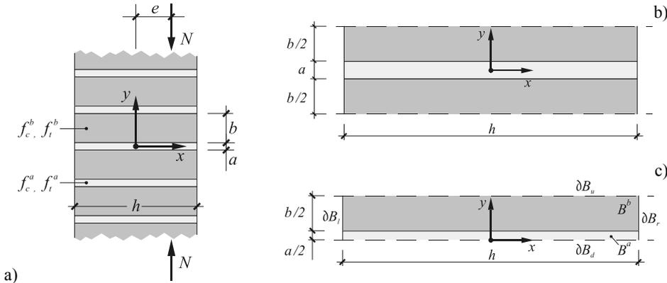
Figure 1. a) Eccentrically compr. column; b) unit cell; c) representative volume element.
