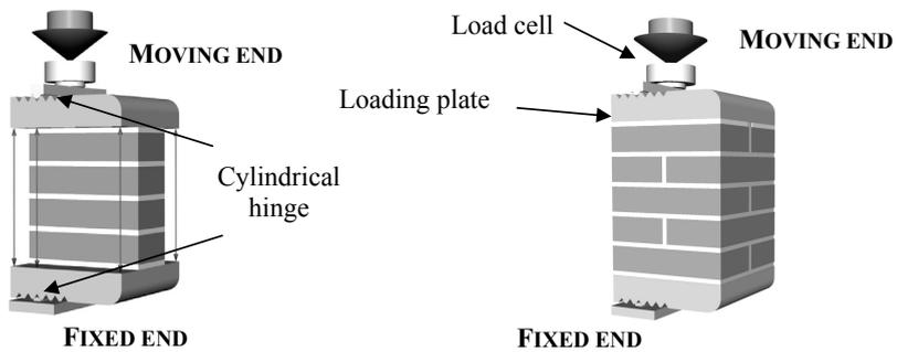
Figure 5. Test setup
