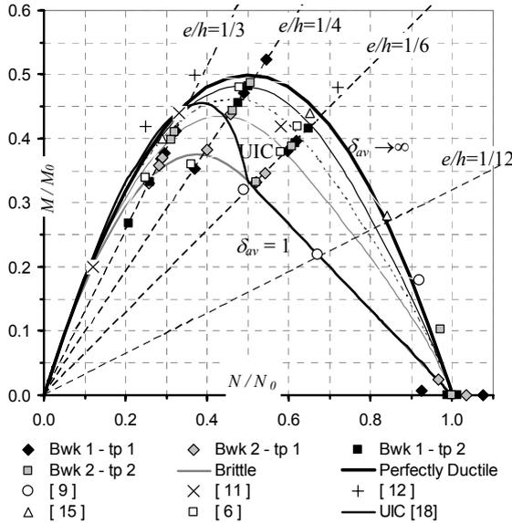
Figure 8. Limit domain of the NTR-EPP model and experimental data in the  $N/N_0$ - $M/M_0$  plane
