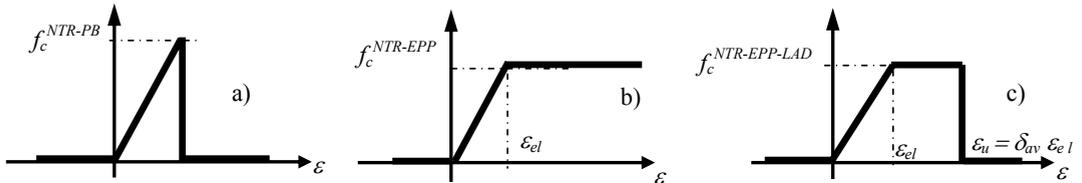
Figure 9. Stress-Strain relationships; a) NTR-PB, b) NTR-EPP; c) NTR-EPP-LAD models
