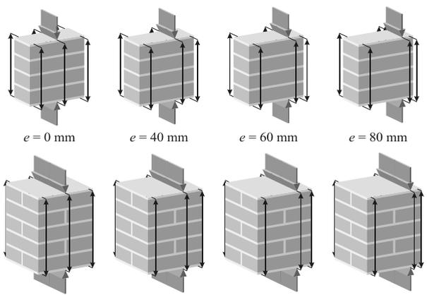
Figure 3. Tested specimens (Dimensions in mm)
