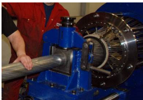
Fig. 3. Full Locked Coil Rope Manufacture. Final z-shaped layer on a 100mm rope.
