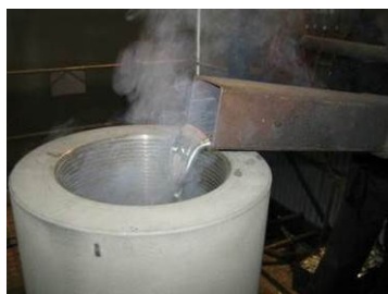
Fig. 7. Socketing of an adjustable open socket with hot metal.
