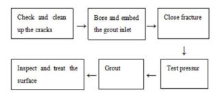
Fig. 8. The process of pressure grouting.
