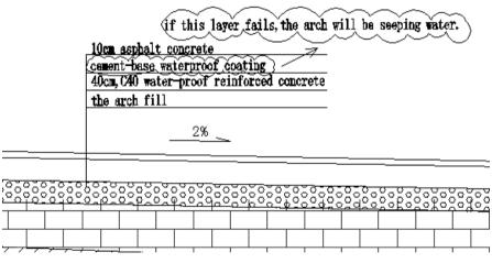
Fig. 6. The schematic diagram.
