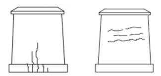
Fig. 5. The abutment cracking.
