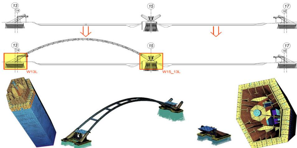
**Fig. 7.** Chart and visualisation of a global and detailed calculation model for the bridge and head section no. 13 for assembly phase: placing arches of a bay 13-15 on assembly tables.
