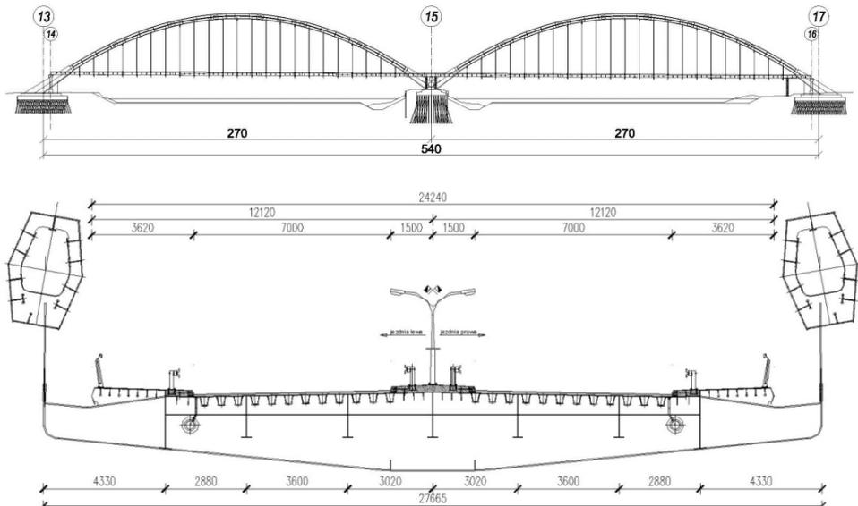
*Fig. 1. Chart and cross-section of arch bridge over the Vistula in Torun.*
