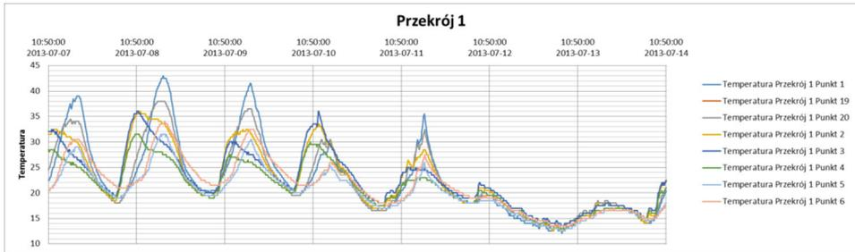
**Fig. 10.** Chart of temperature changes within steel structure in a cross-section 1-1 of a head section no. 13 at the assembly phase: suspension and joining with the remaining platform segment JMP6 of a bay 13-15.
