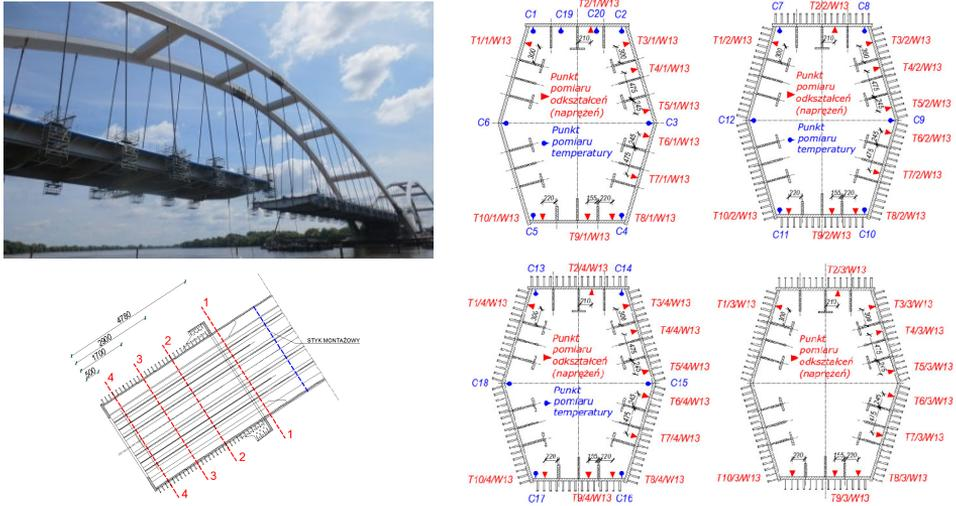
Fig. 8. General view of the structure after suspension of platform segment JMP6 of a bay 13-15; layout of cross-sections and measuring points of a head section no. 13.
