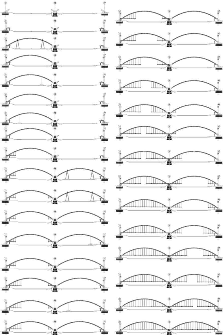
*Fig. 3. Phases of assembly of arch bridge over the Vistula in Torun.*
