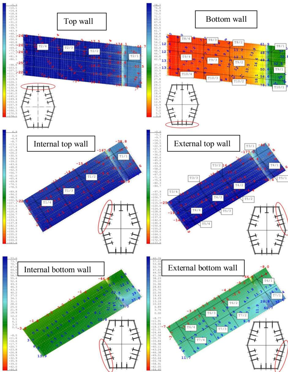
**Fig. 11.** Maps of theoretical values of stresses  $\sigma$  [MPa] in a steel part of a head section no. 13 for the assembly phase: suspension of a platform section JMP6 of a bay 13-15 (considering the influence of temperature of the structure at the moment of measurement).
