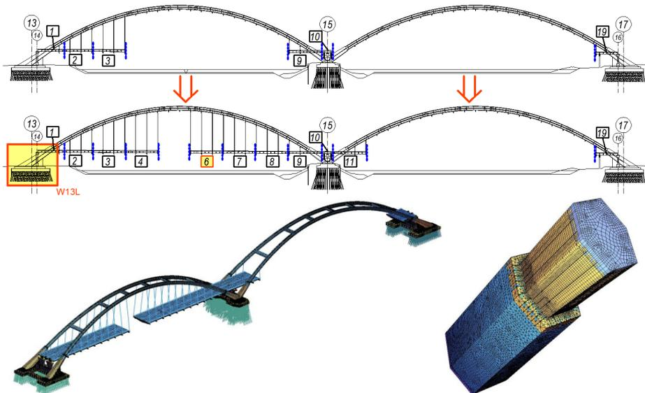
Fig. 9. Chart and visualisation of a global and detailed calculation model for a bridge and head section no. 13 for the assembly phase: suspension of a platform segment JMP6 of a bay 13-15.
