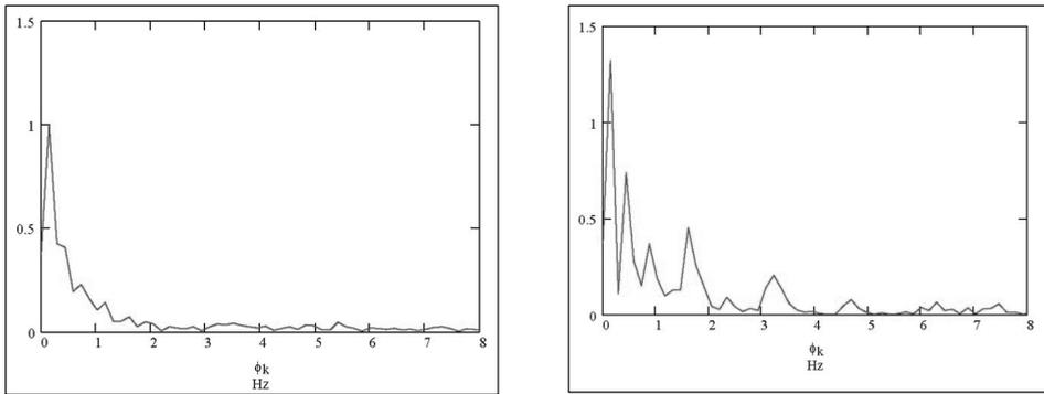
Figure 12: Fourier spectra (left) and wavelet spectra (right) of a same signal. Wavelet spectra allow an easier detection of resonance frequencies
