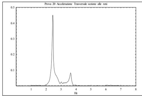
Figure 14: Fourier spectra of a transversal accelerogram
