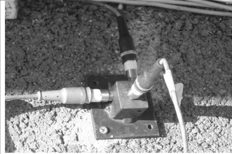
Figure 6: HBM inductive accelerometers
