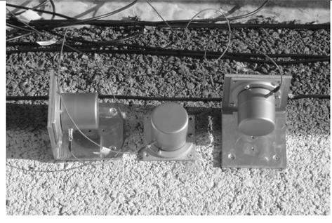
Figure 7: PCB piezoelectric accelerometers
