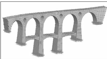
Figure 9: the finite element model of the bridge
