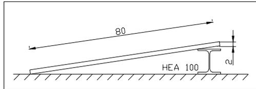
Figure 5: step geometrical features
