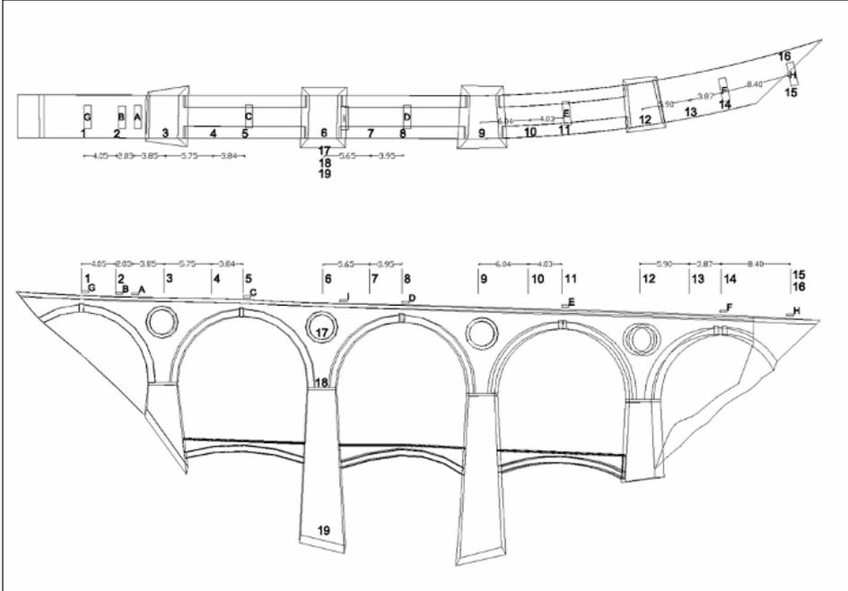
Figure 3: Outline of the way the instruments were placed. Letters denote the step position, numbers denote the accelerometers positions.
