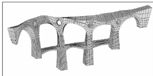
Figure 10: the second mode of vibration
