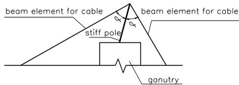
Fig.3 FE model in saddle
