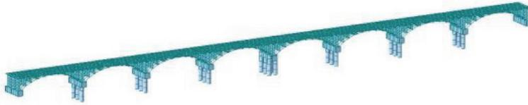
Figure 3: The FE model of Wuli bridge
