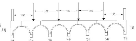
Figure 1: Transversely eccentric arrangement of two vehicles
