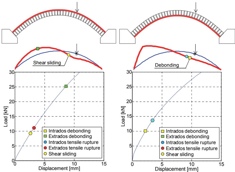
Figure 3: Collapse configurations and load-displacement curves of strengthened arches under concentrated load at 3/4 span: extrados (a) and intrados reinforcements (b)
