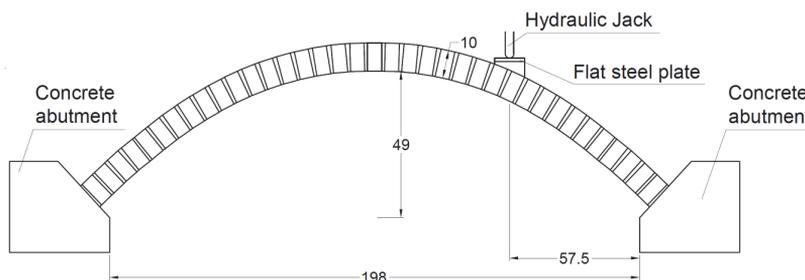
Figure 2: Strengthened masonry arch tested in laboratory [3]
