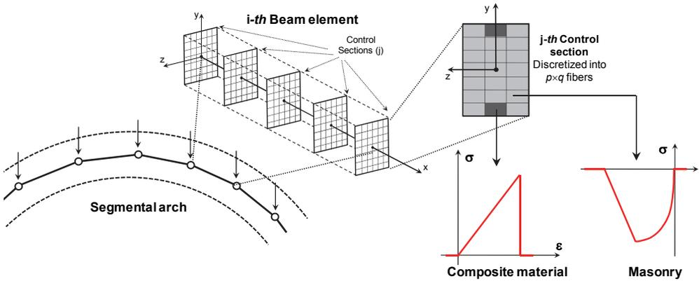
Figure 1: The fibre beam based modelling approach
