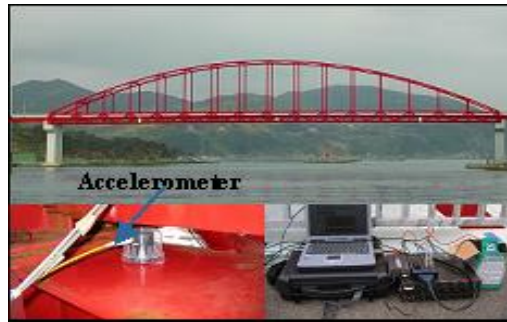
Figure 1 : Ambient vibration measurement on Kabashima Bridge
