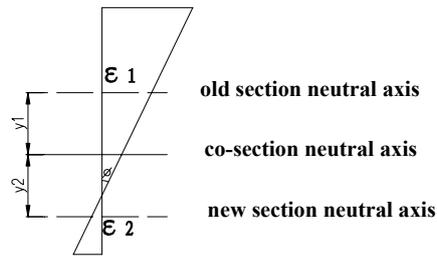
Figure 3 : The strain drawing of Co-section
