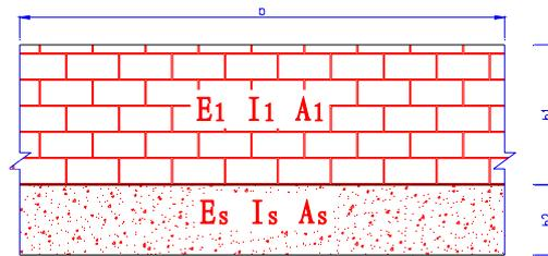
Figure 2 : The structural drawing of the widening section method for reinforcing arch ring
