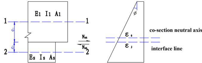
Figure 4 : The calculation sketch drawing of self constraint internal force of arch ring shrinkage
