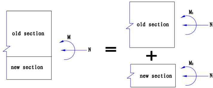
Figure 1 : The sketch drawing of section internal force distribution
