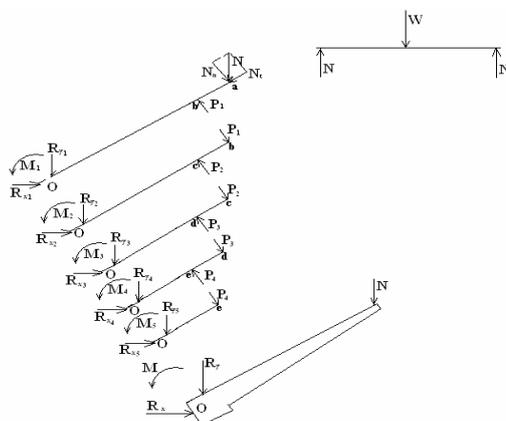
Figure 5: Components Subjected to Loads of Oblique Stacked Beam Arch Bridge of Baling
