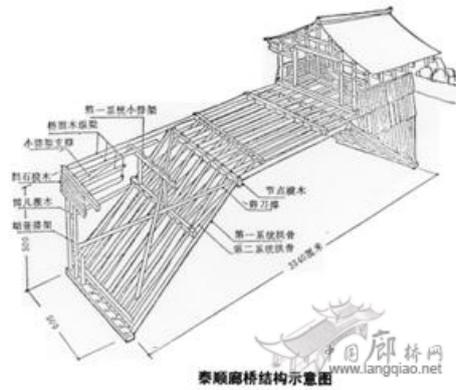
Figure 7: Diagram of the Structure of Taishun Gallery Bridge
