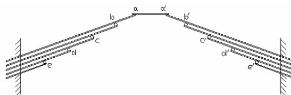
Figure 4: Structure of Oblique Stacked Beam Arch Bridge of Baling
