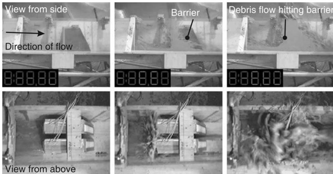
Figure 3 : Side view and view from above of the used debris flow impact measurement test set-up (Hübl & Holzinger 2003)
