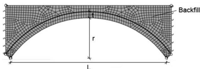
Figure 4 : FE model of a simplified arch bridge (Becke, 2005)
