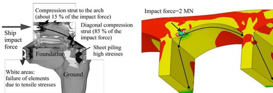
Figure 2 : Examples of the structural behaviour under impacts (left against the pier, right against the arch itself) (Proske and Hübl 2007)
