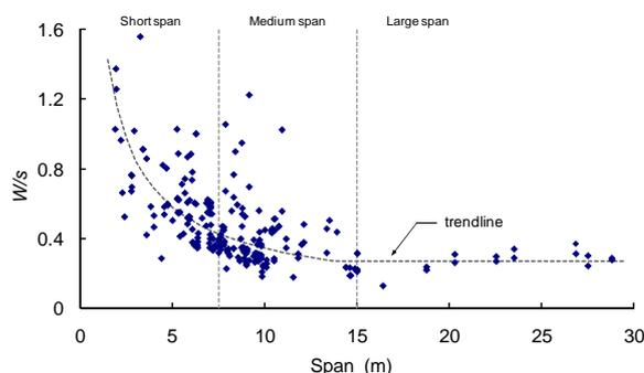
Figure 2 : Relation between the span and the width to span ratio.
