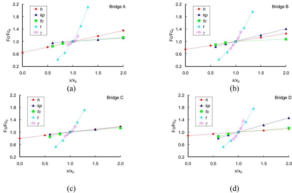
Figure 1: Non-dimensional relationship between the load factor and the 5 parameters considered for: (a) semi-shallow short span bridge (type A); (b) deep short span bridge (type B); (c) semi-shallow medium span bridge (type C); (d) deep medium span bridge (type D). The variable  $x$  is referred to any of the five parameters considered.
