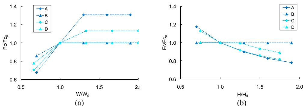
Figure 4 : Non-dimensional relationship between the load factor and: (a)width of piers, (b)height of piers. A-D indicate the reference bridge being considered
