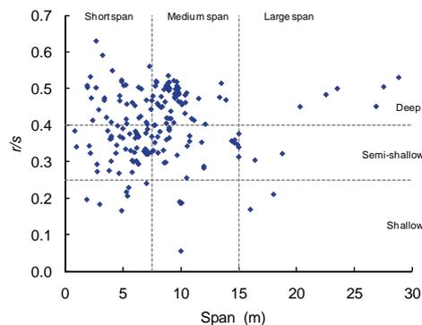
Figure 1 : Relation between the span and the rise to span ratio.
