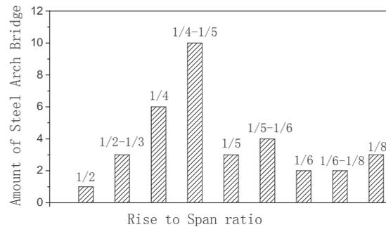
Figure 3 : Ratio of rise to span arrangement
