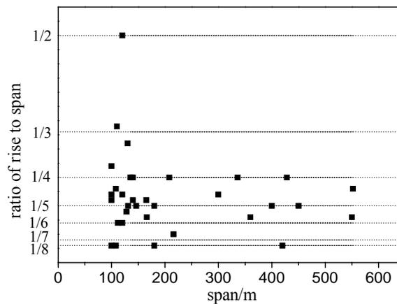
Figure 4 : relationship between ratio of rise to span and span
