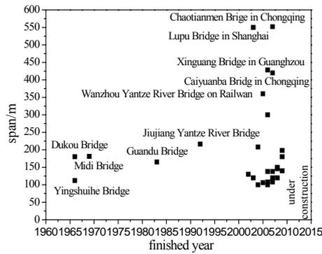
Figure 1 : span and finished year of steel arch bridge
