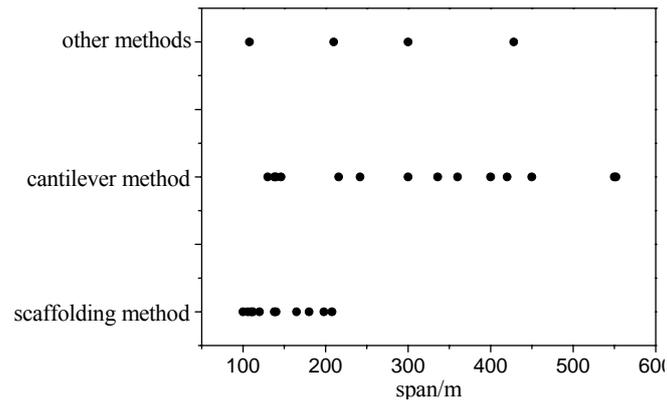
Figure 5 : relationship between construction method and span
