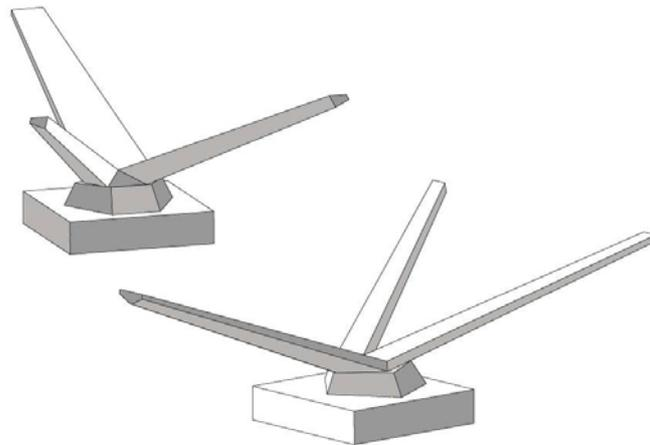
Figure 4 : Piers' Tripod perspective
