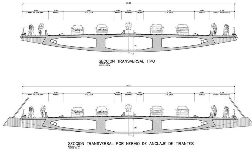
Figure 10 : Deck's transversal section
